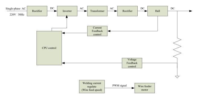
This equipment has an excellent volt-ampere characteristic with the relation between the rated loading voltage U2 and welding current I2 is as follows: **U2=14+0.05l2(V)** (see diagram below)
